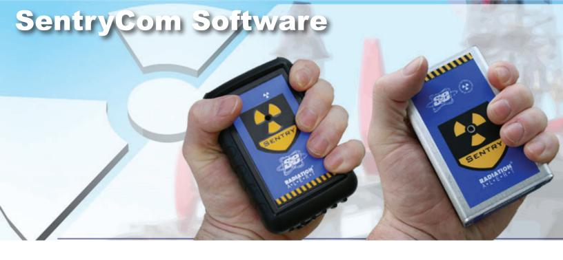
The Windows® based SentryCom Software enables you to set the values for dose and dose rate alarms and warnings, set the Cal Factor, and the data logging frequency. It also allows the user to download the accumulated exposure data, which includes time and date stamp, exposure, and power cycle identifiers for analysis. The data is stored in a convenient delimited text file for use with a spreadsheet program.
